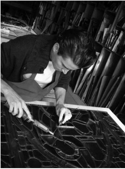
Daniel Maloney soldering copper ties to a panel.
