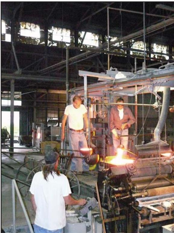
*Molten glass is hand poured into the rolling machine, which will form it into a sheet of glass.*
